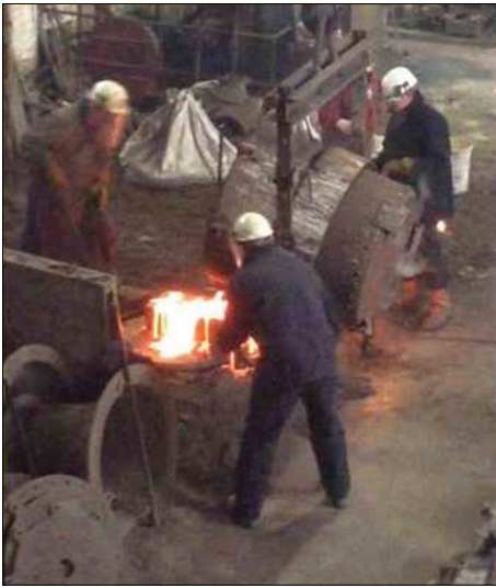
The tenor being cast on 20th March 2013 at the John Taylor Bell Foundry, Loughborough
